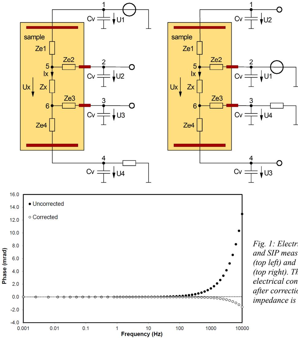
*Fig. 1: Electrical models of the sample and SIP measurement system for normal (top left) and reciprocal measurements (top right). The phase of the complex electrical conductivity of water before and after correction for the electrode contact impedance is also shown (bottom).*
