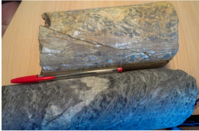
Fig. 3: MFT80 core drilling. Oxidized (top, from 25 m depth) and unaltered (bottom) schist samples.
