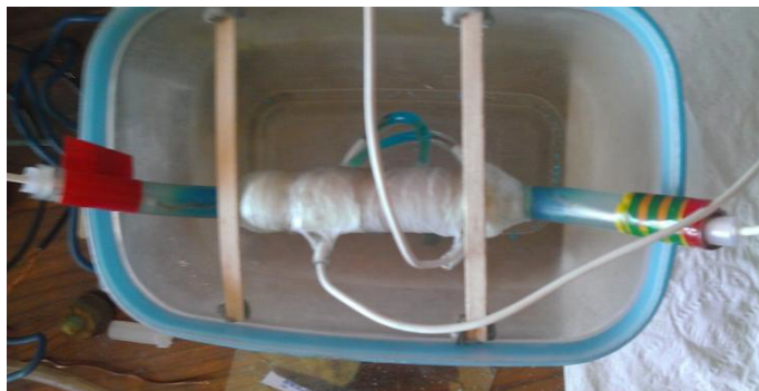
Fig. 1: Installation for IP measurements, the sample is in the centre, in the plastic tube.
